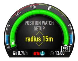
Rotate the Jog wheel to select the monitoring radius; click to confirm.
